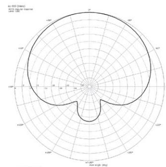
Polardiagramm @ 1 kHz
