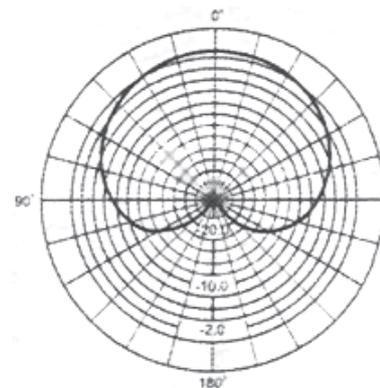
Polardiagramm @ 1 kHz
