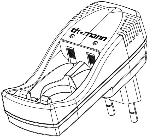
The battery charger 2 set is a plug-in battery charger to rapidly charge batteries with 2 loading slots usable independently from each other.
