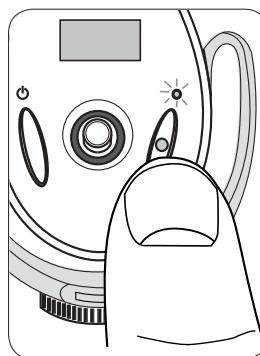
● **Record:** Press the record button to begin recording. The LED indicator illuminates while recording. Pressing record always creates a new track, unless resuming a paused recording.
