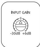
**Input Gain:** Sets the level of the input signal before it is amplified.
