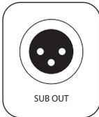
**Sub Out:** This balanced XLR output sends the low-frequency signal from the lowpass filter to a second Temblor T10. When connecting a second T10 to this output, set its Low Pass Filter control to its highest setting.
