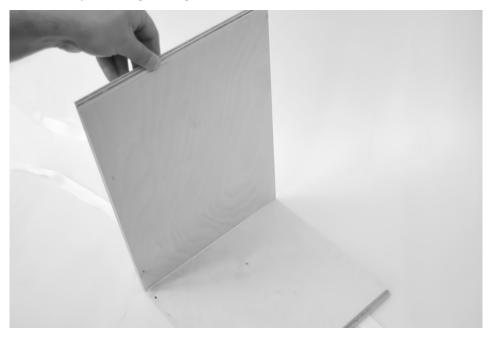
After you have glued the two side panels to the floor panel check them for flushness and glue the top plate in the same way.
