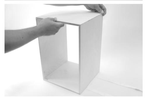
Slide the supplied cardboard angle template centrally into the body to create a straight angle.
