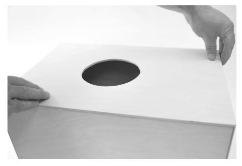
Put the pressure plate on the back panel, check the edges for flushness and press the pressure plate briefly.
