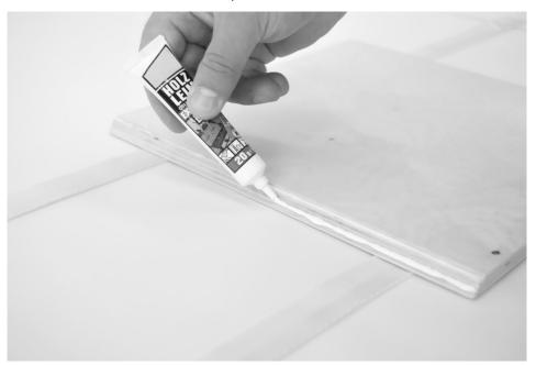
Insert the side panels into the milling edges of the floor panel. When installing the side panels and gluing them with the floor panel, ensure that the edges line up precisely.
