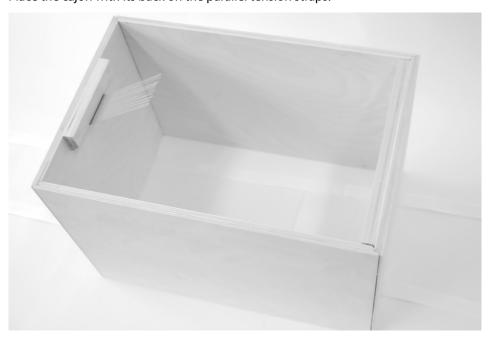
Carefully apply the express glue along the body edges, snare and bottom strip.
