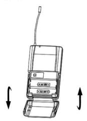
The battery compartment of the UHF pocket transmitter is located on the back of the device.
