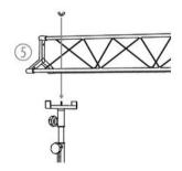
**5.** Attach the mounted truss beam and fix it in the desired position with the wing nuts.
