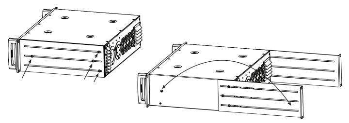
\* NOTE: Please use the screws which are provided. If screws must be obtained elsewhere, do not use screws longer than 5/16 of an inch. Screws longer than 5/16" may contact internal components rendering the unit inoperable.
