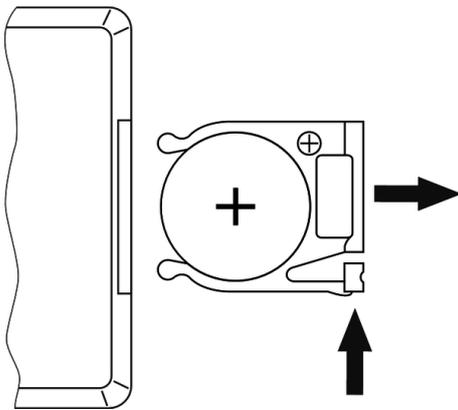
When shipping, the battery is already installed in the remote and protected against discharge by a transparent plastic foil. Remove the plastic foil prior to first use.
