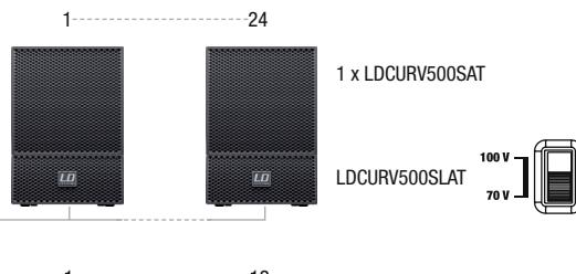
2 x CURV 500 Satellit pro SmartLink Adapter 70V = Menge maximal 12 SmartLink Adapter (12 x 40W = 480W max.)
