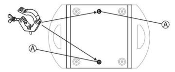
A Quick lock openings for Omega brackets
