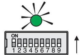
As soon as the fog machine receives DMX control signals, the green DMX indicator lights up and the machine can be operated with the DMX controller.
