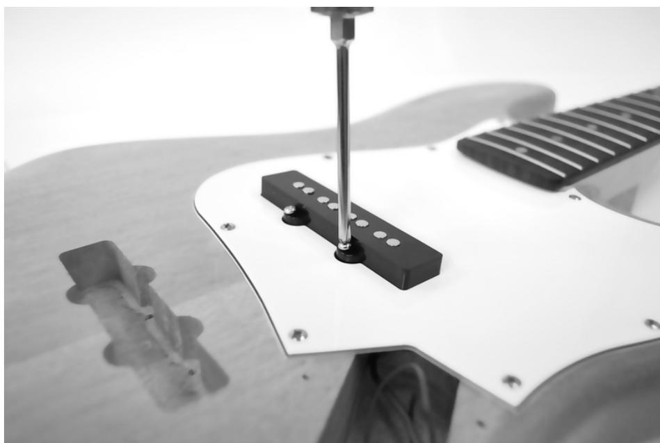
As illustrated, run the cable connector for the bridge pickup from the recess for the pickup into the cable channel and as far as the recess for the potentiometer plate.
