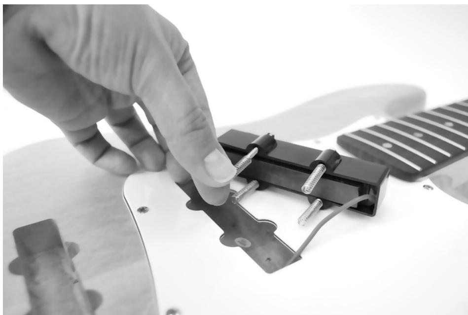
Screw the neck pickup into the recess for the pickguard using the supplied screws.
