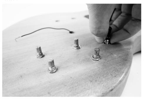
Screw the switch to the body surface with the plastic cover provided, a washer and a hex nut. The neck pickup is generally activated with the switch in the upper position, and the bridge pickup in the lower position. This configuration can be changed at any time simply by swapping the two connectors.
