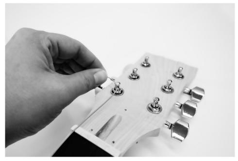
Then tune each string in turn to the correct pitch. You can using a tuner or a pitch pipe as a reference. Please note that the string tension will still drift and the guitar will need to be retuned a few times before the strings are played in.
