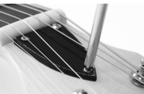
Screw the cover for the truss bar onto the header headstock.
