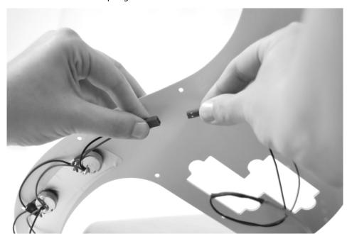
Connect the connector to the connector for the potentiometers and output jack which is mounted on the pickguard.
