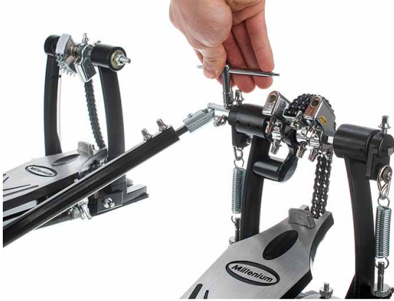
Step 2: Fix the cardan shaft on the left bass drum pedal
