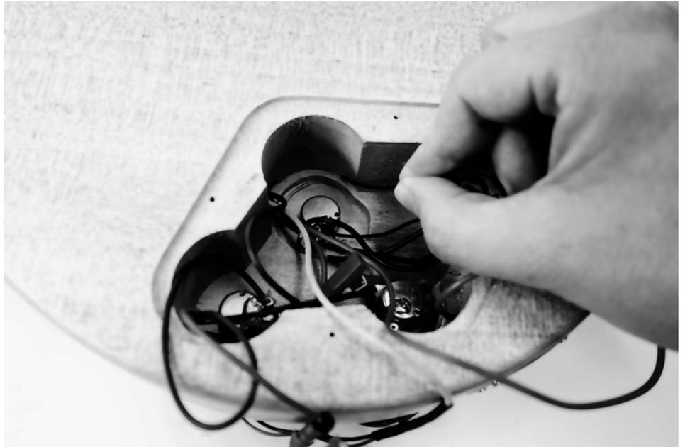
Pull the cable far enough out of the hole that there will be sufficient contact with the metallic surface when the tailpiece is installed. Earthing the strings reduces noise (humming).
