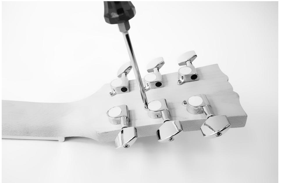
Turn the neck and fasten all the machine heads finger-tight to the front of the headstock with the washers and nuts provided.
