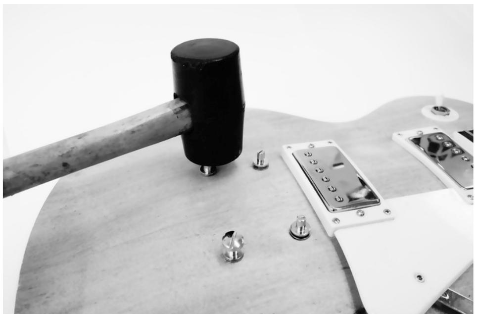
Place the tailpiece and the bridge on the fastening bolts. These two components are still loose, and will only be fastened when you string the guitar.
