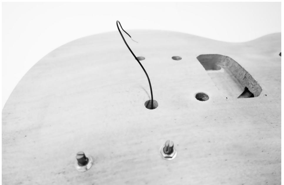
Thread the pickup cables through the channels from the front opening into the back opening. The neck pickup is somewhat flatter and is inserted into the opening nearer the neck of the guitar. Insert the somewhat taller bridge pickup into the opening closer to the bridge.
