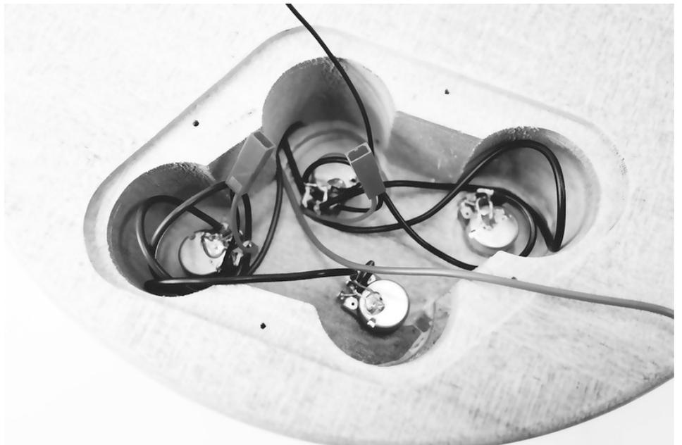
Thread the cable for the string earthing (after stripping the insulation, and without the connector) through the channel from the opening in the back into the hole to fasten the tailpiece.
