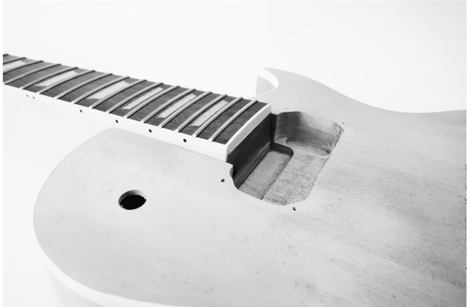
Turn the guitar over and position the neck plate over the four bolt holes at the rear of the body, then screw the four wood screws provided through the neck plate, body and pilot holes in the neck until everything fits tightly.
