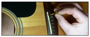
8. Guide the white pin up through the high E string hole from the inside and secure the jig by moving the golf tee to the G string hole from the outside and finding the oblong hole in the jig. This will align the jig exactly as was done in step 3, during the practice run.
