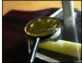
10. Once the pickup is in place, apply pressure to the jig/ pickup while you slowly count to 30 to allow the glue to set. Release the pressure, but **leave the jig in place for another 5-10 minutes** to allow the glue to cure before continuing.
