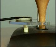
We recommend that you do a test run without using the glue at this point to practice finding the right position for the jig inside the guitar.
