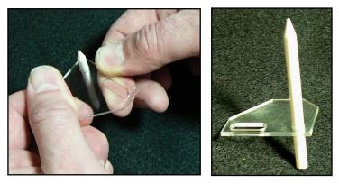
The pin should fit very snugly – you may have to use some force (or even file it down a bit) to press it into the hole. If the pin fits too loosely, please use some superglue to secure it. Wipe off excess glue and let dry.
