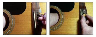
9. Once you confirmed that the procedure works as intended, you can apply glue the golden side of the pickup and glue it in. Please ensure that the putty still holds the pickup firmly in place after the trial run. Use a fresh piece of putty if necessary.
