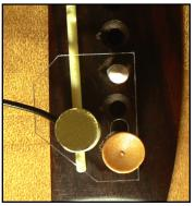
13. Here is how the finished result will look inside the guitar. You can use a mirror and flashlight to check that the position of the pickups is correct.
