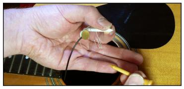
7. Move the jig inside the guitar through the soundhole. Stick the golf tee into the high E string hole from the outside with your other hand and try to feel it protruding to the inside with the thumb or index finger of your jig hand. This process helps you identify the correct pinhole on the inside.
