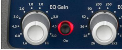
The mpressor rack comes with the Niveau Filter EQ, generating very useful and unique filter curves with a set of just two controllers. This feature could not be implemented into the 500 series module because the space was just not available on the front panel.
